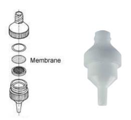
The GVS Swinney 13 mm filter holder is optimized for small volume (1-5 mL) particulate removal from fluids dispensed with a syringe. The holder is resistant to alcohols, esters, ethers, glycols, aromatic hydrocarbons, halogenated hydrocarbons, ketones, oils, photoresists and many other chemicals. Although suitable for most weak acids and bases, we recommend that you test for compatibility with acids.
