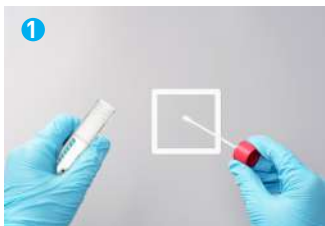
Fix the area to be tested using a sterile template plate.
